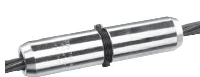
The use of couplers makes it possible to save wastage of prestressing steel in pretensioning work. They are available for joining together wires/strands of identical or of differing diameter.
