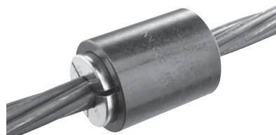
Open or A-Type grips are the least expensive, most robust and most commonly used type of grip. They are easy to handle and to clean and are generally used at the stressing end of the casting bed. When used with single-wire stressing jacks with hydraulic lock-off facility open grips have the advantage that pull-in losses are reduced to an absolute minimum. Also on detensioning they are very easy to handle. Open grips are also often used as post-tensioning grips.
