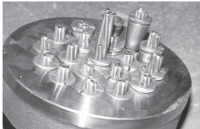
Anchor plate with compression wedges
